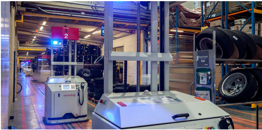
Automated guided vehicles: Automating transport routes saved AMAG four full-time jobs.
